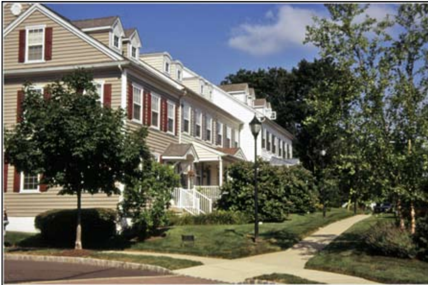
A network of shaded sidewalks provides access throughout the Lantern Hill TND. This particular grouping of houses fronts on the sidewalk, not on a street. The alley to the rear of the houses provides access to off-street parking. Lantern Hill uses a housing court concept in parts of the TND.
