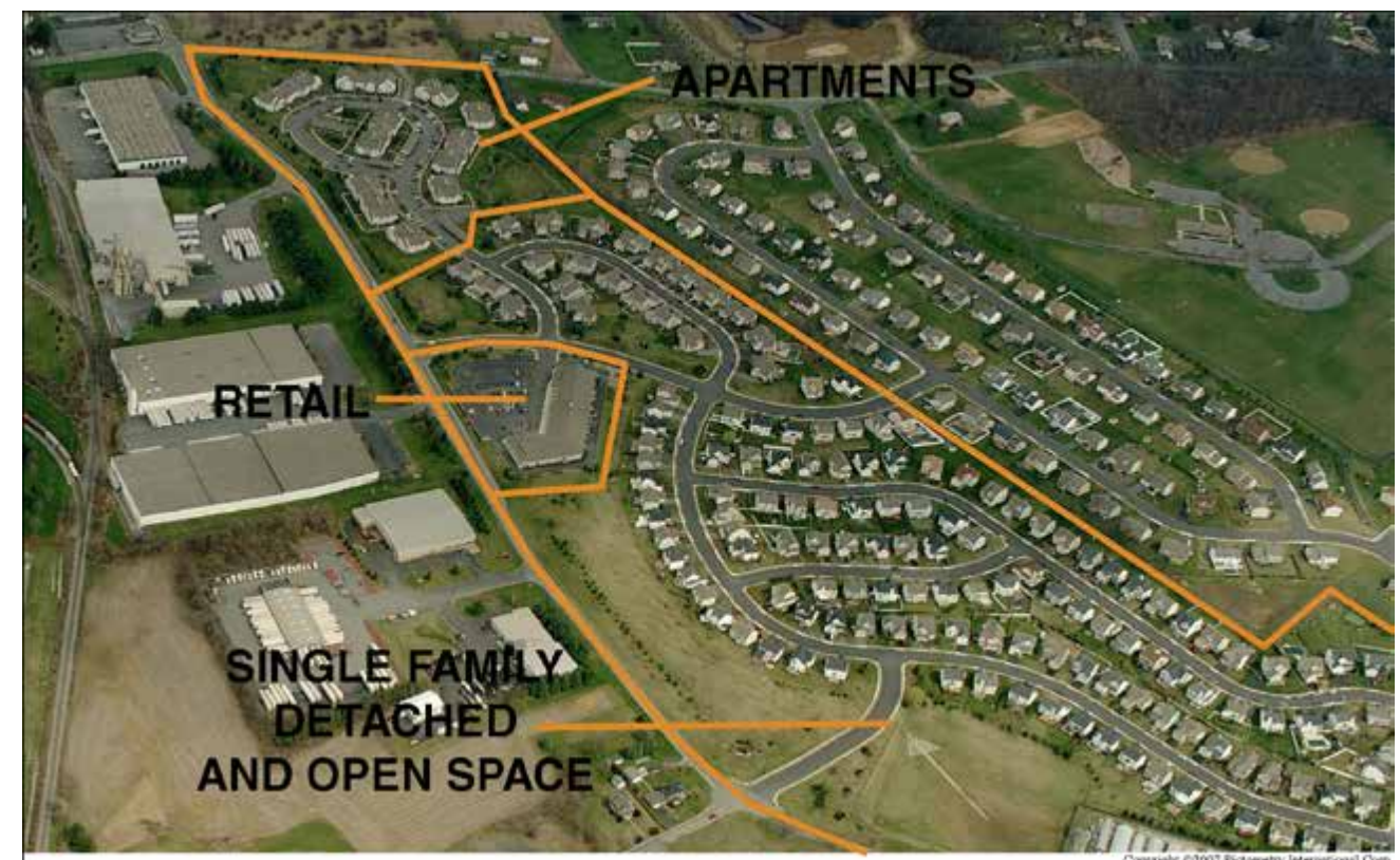
Olde Towne is a mixed use development in Upper Macungie Township that includes single family detached dwellings, apartments and retail development. Each use is compartmentalized on a different part of the site.
